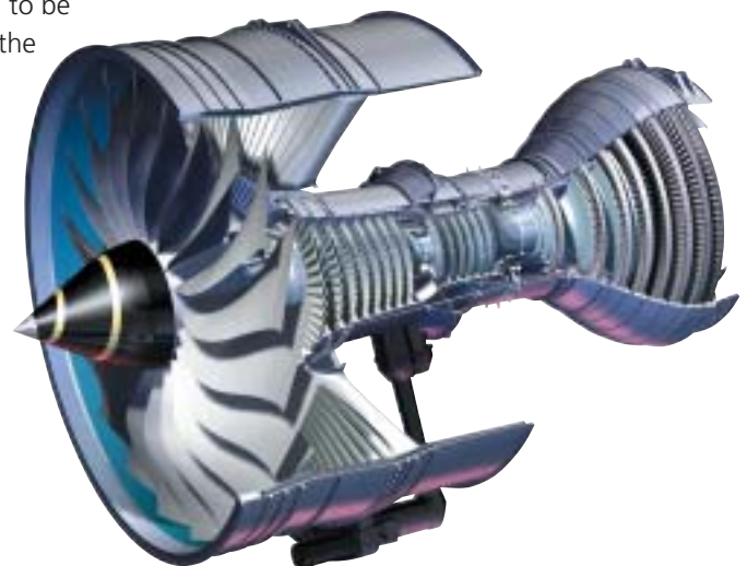
High-performance Rolls-Royce Trent 1000 engine
