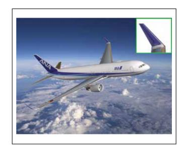
Manufactured by Airline Partners Boeing, each winglet is 3.4m long, 4.5 m wide, and will extend the length of each wing by 1.65m. By improving the aerodynamics of the wing, ANA expects to make an efficiency gain of 5%, or a saving of 2,100 tonnes of CO<sub>2</sub> per annum for each aircraft.
