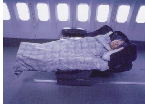
In 1996, ANA began installing new first-class seats on 747-400 and 747-LR aircraft. The seats are spaced 83 inches apart and recline to a completely flat position.
