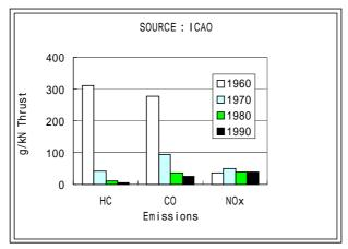
Fig.3-1 Progress of Engine Emissions
