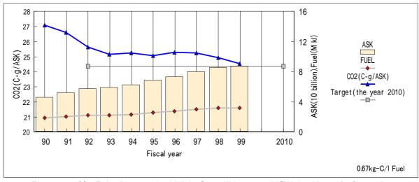
Fig.5-3 CO2 Emission per Available Seat-Kilometer (ASK) by Aircraft Operation
