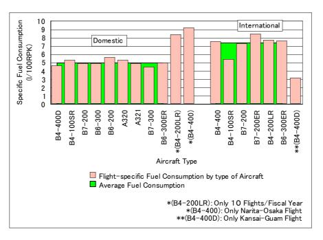
Fig.5-6 Flight-specific Fuel Consumption by Type of Aircraft in 1999
