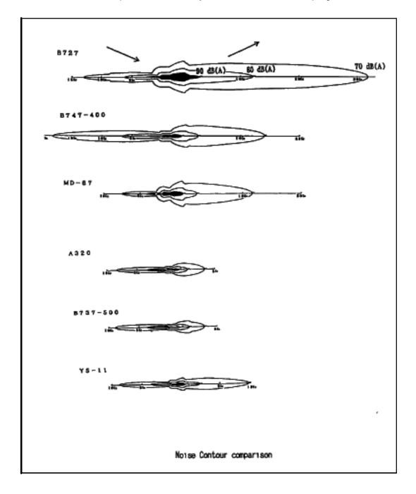
Fig.2-3(1) Noise Contour comparison
