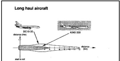
Fig.2-3(2) Noise Contour comparison (Sources: Airbus Industries)
