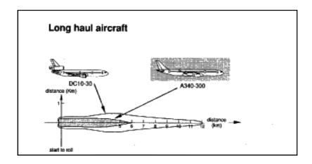
Fig.2-3(2) Noise Contour comparison (Sources: Airbus Industries)
