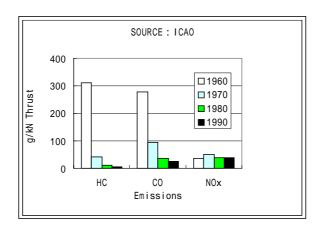
Fig.3-1 Progress of Engine Emissions
