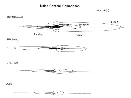
Fig.2-3 (1) Noise Contour comparison
