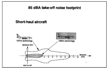
Fig.2-3(2) Noise Contour comparison (Sources: Airbus Industries)
