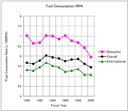
Fig.5-4 Actual Fuel Efficiency
