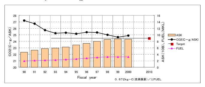
Fig.5-3 CO<sub>2</sub> Emission per Available Seat-Kilometer (ASK) by Aircraft Operation
