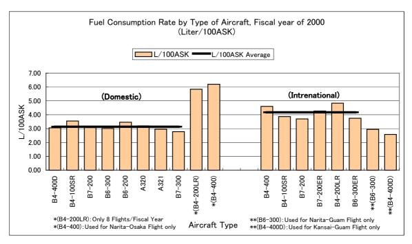
Fig.5-6 Flight-specific Fuel Consumption by Type of Aircraft in 2000
