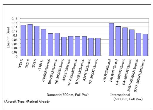
Fig.5-5 ANA Fleet Fuel Efficiency Comparison
