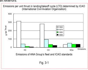
past 30 years, but NOx has not been reduced to as great an extent. This is because pressure and temperatures in combustion chambers have been raised in order to improve the combustion efficiency of jet engines.
