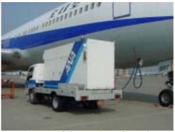
Low-noise type AC Electrical Power Supply Car
