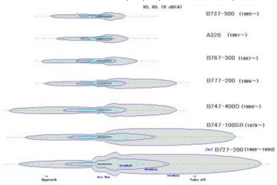
Fig. 4-3 Comparison of noise contour by aircraft type
