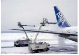
Low-noise type de/anti-icing vehicle (New Chitose Airport)
