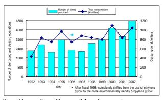
of dry, midwinter snow at Chitose Airport), followed by coating with an anti-freezing agent. The ANA Group has completely shifted its use of anti-freezing agent to propylene glycol (an environmentally friendly substitute that is not subject to the Japanese PRTR Law), and has made efforts to develop better equipment and to improve work procedures so as to reduce the amount of anti-freezing agent used.
