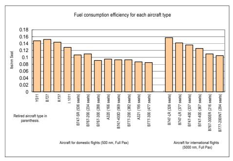
Fig. 2-5 Fuel consumption efficiency of each aircraft type
