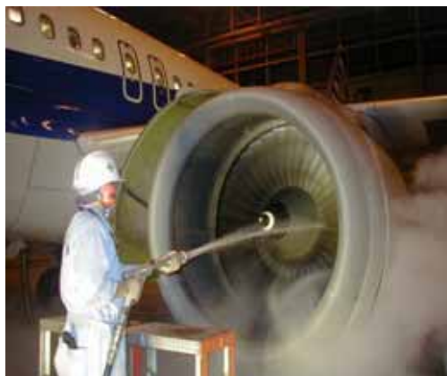
This picture shows a trial of an engine wash procedure for the A320 aircraft. Special equipment is employed in the engine wash procedure for the B777.
