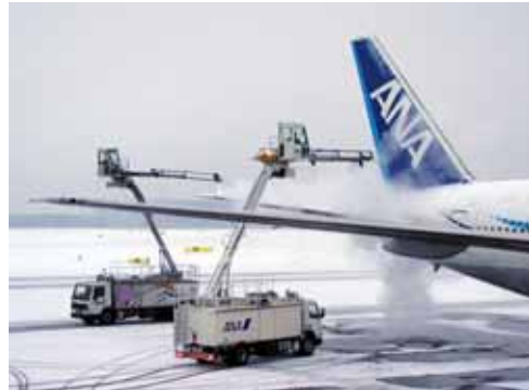
State of the Art de/anti-icing vehicle fleet, low noise blower equipped (Front)
