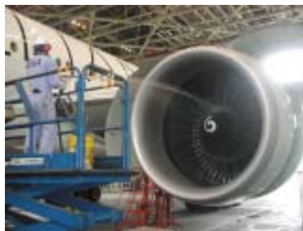
Washing the engine compressor
