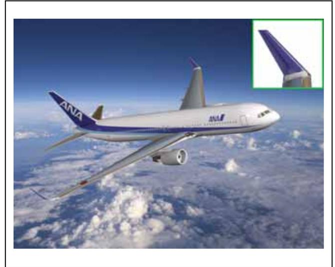
Manufactured by Airline Partners Boeing, each winglet is 3.4m long, 4.5 m wide, and will extend the length of each wing by 1.65m. By improving the aerodynamics of the wing, ANA expects to make an efficiency gain of 5%, or a saving of 2,100 tonnes of CO<sub>2</sub> per annum for each aircraft.
