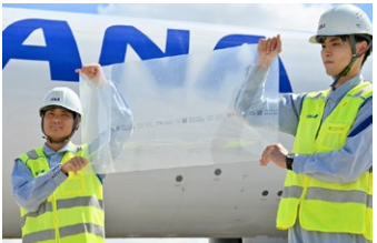
AeroSHARK riblet film
