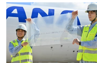
AeroSHARK riblet film
